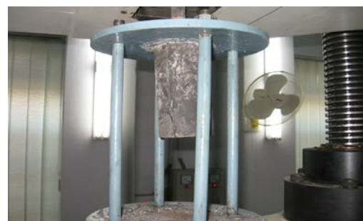
Fig.10. Formation of longitudinal splitting cracks
