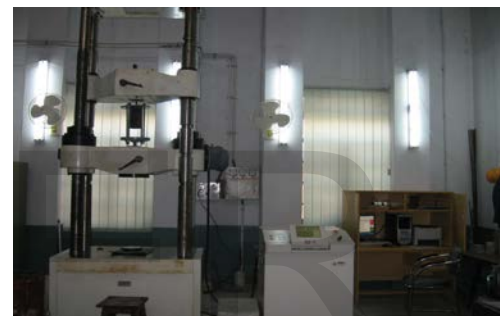
Fig.9. Compression test in UTM
